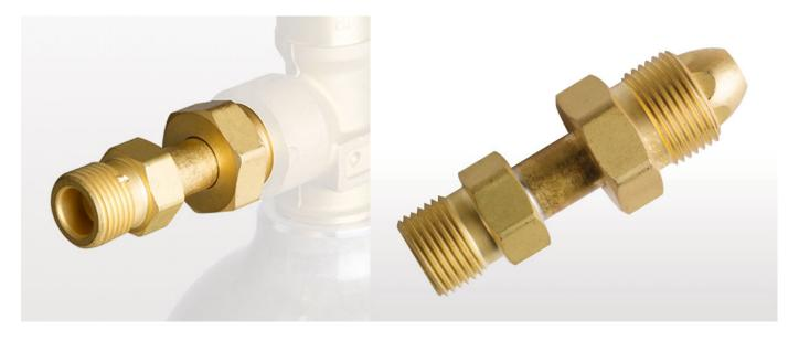
Adapter fitting quickly converts Nitrogen CGA 580 cylinder to compressed air CGA 346 for filling with compressed air. Cylinders are to be filled to 2000 psi on a 2216 psi filling system with Nitrogen or compressed air.
