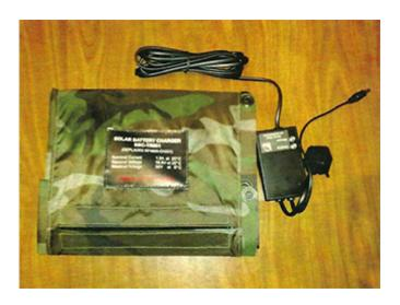
BC-LI1 - Charges BB2590/U Li-Ion batteries BCNI1 - Charges BB590/U, BB390/U or ALI116 batteries
